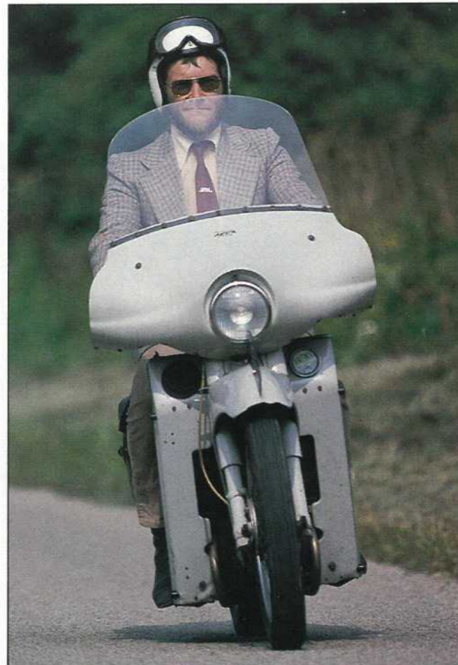
Broad Avonair fairing fitted to the LE offers better protection than the slimline Vogue. Top speed for both models is a beady 60mph.
