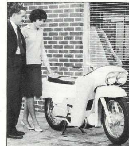
Velocette Ltd announced the Vogue in 1963. The GRP body was made by Mitchenall Brothers.
